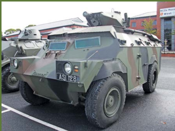
Above: front left view of the Timoney Mk VI APC (armoured personnel carrier) fitted with a TLI 127 turret.
