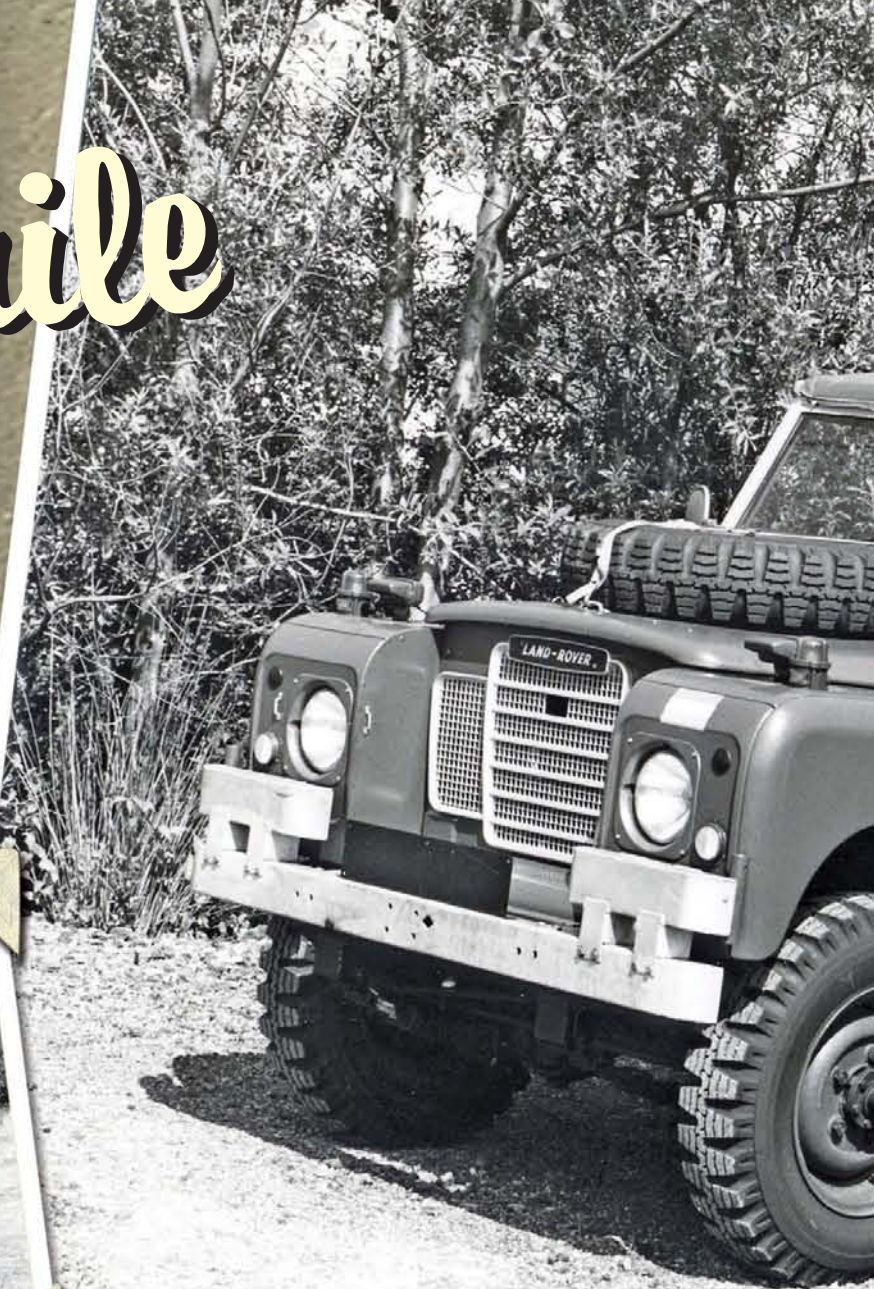
Left: pictured before allocation of its Dutch number-plate, this Lightweight is wearing the locally manufactured NEKAF tyres that caused so much difficulty. The S painted on the bonnet indicates that the vehicle was electrically suppressed.
