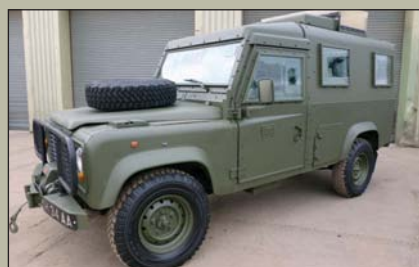
Defender 110 LHD fitted NP Aerospace CAV 100 VIP Armoured body, 300 TDI turbo diesel engine, R380 Gearbox, power steering, front + rear antiroll bars, Composite body with steel doors, sliding top cover hatch, air conditioning, etc Mileage from 39,000, Guide price from £15,000 (2 Available)
